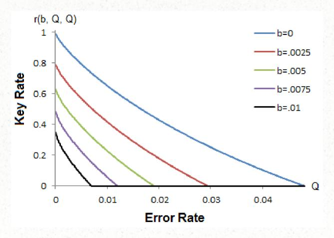
Q is the probability that a |i> flips to a |1-i>  $Q_x$  is the probability that a |+> flips to a |-> Above, we consider the case when Q =  $Q_x$
